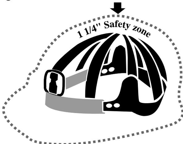
As with devices designed to protect eyes, the design, construction, testing, and use of protective helmets must meet standards established by ANSI. Protective helmets purchased after July 5, 1994, must comply with ANSI Z89.1-1986,\* whereas, those purchased before this date must meet the ANSI Z89.1-1969 standard.
