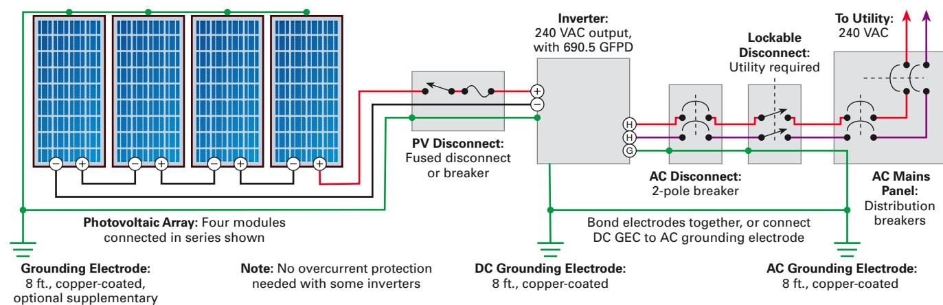
building slab is used as the grounding electrode, a #4 (21 mm<sup>2</sup>) GEC is required.
